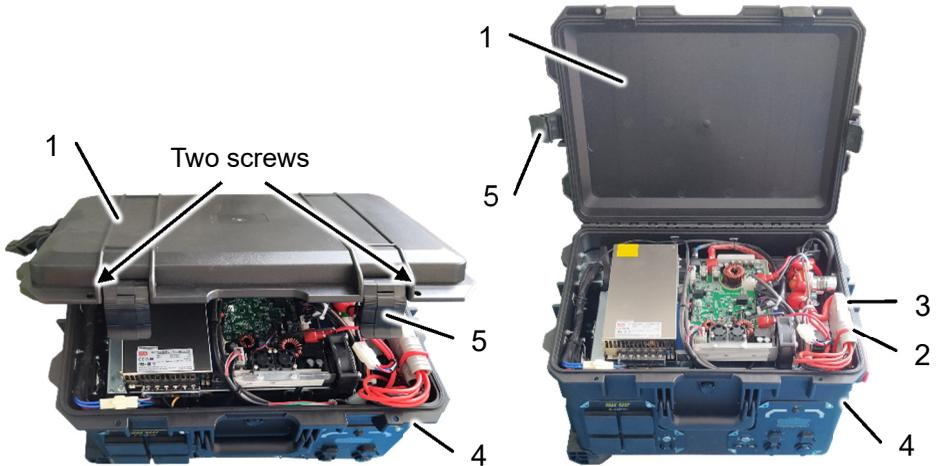
**You need to connect the battery connector 2 before charging or using the power station:**
